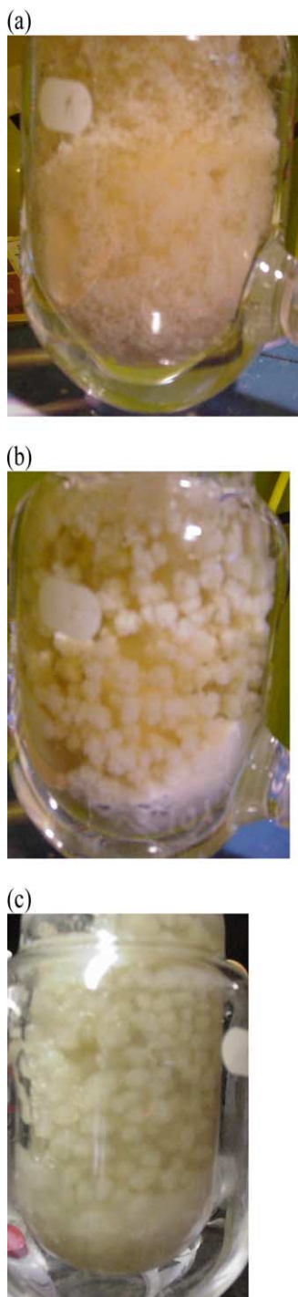
Fig. 10. (a) Slurry polymerization with 100% styrene (10 min). (b) Slurry polymerization with 100% styrene (45 min). (c) Slurry polymerization with 100% styrene (55 min).
