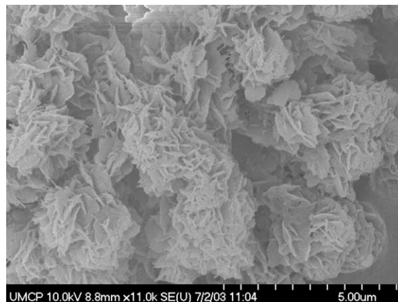
Fig. 2. SEM image of embedded catalyst (sPS prepolymer). (a) Slurry polymerization at 10 vol% styrene, 30 min; (b) 60 min.
